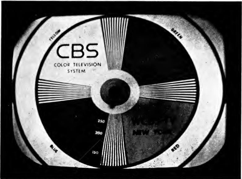
Fig. 11. Test pattern, transmitted with system flat to 10 mc, uncrispened.
